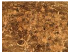
Figure 2. Photomicrograph of a thin section of the brecciated limestone from Nahavand.
