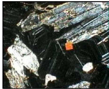
Figure 6 : microscopically picture garnet, wollastonite and clinpyro xene
