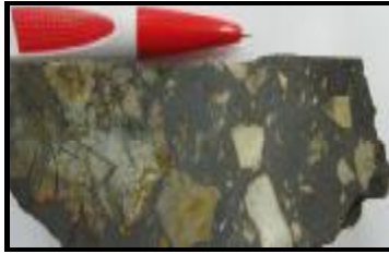
Fig. 5: Hydrothermal breccias. A cement of magnetite surrounded floated fragments of host rock.
